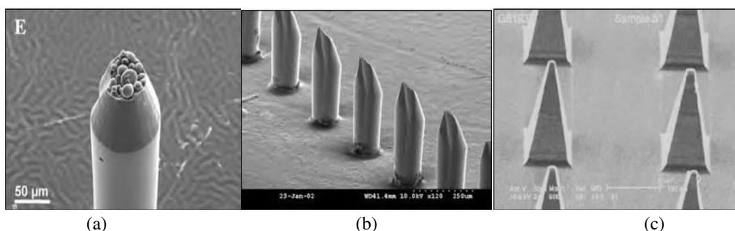
Fig. No. 04: <sup>[2]</sup>(a) 3M's Microstructured Transdermal System (MTS). 250  $\mu\text{m}$  long molded polymer needles. (b) Beveled PLGA microneedles inserted through human epidermal tissue *in vitro*. The needles are approximately 400  $\mu\text{m}$  long. (c) Drug incorporated microneedle. The picture shows a cut off tip of a PLGA micro needle incorporating PLA micro particles encapsulating calcein.
