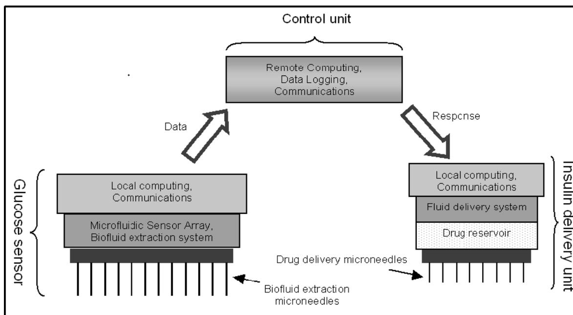
Fig. No. 06: Elements of the prototypical microneedle-based autonomous diabetes therapy system.
