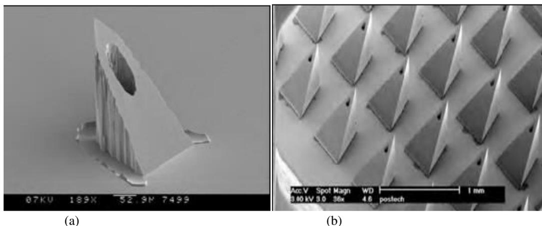
Fig. No. 05: <sup>[2]</sup>(a) 350  $\mu$ m long silicon microneedle by Gardeniers *et al.*, etched by combining DRIE and wet etching. (b) Microneedles made in PMMA by Moon and Lee, using LIGA techniques.
