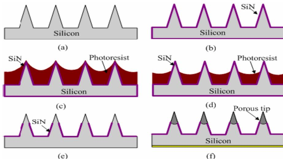
Fig. No. 02: Fabrication schedule of microneedle array with porous tips
