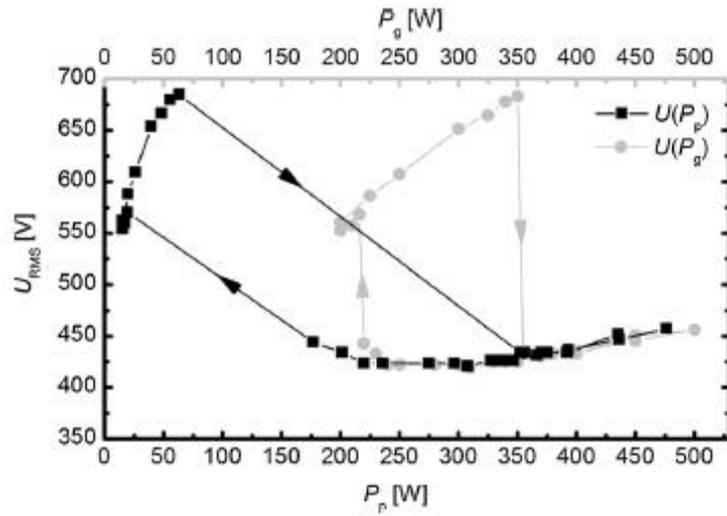
Fig. No. 09: Influence of the resistive antenna heating on the hysteresis for E- and H-mode at 40 Pa (generator power vs. plasma power)
