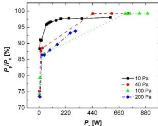
Fig. No. 05: Power transfer efficiency for four different pressures shown as a function of applied power
