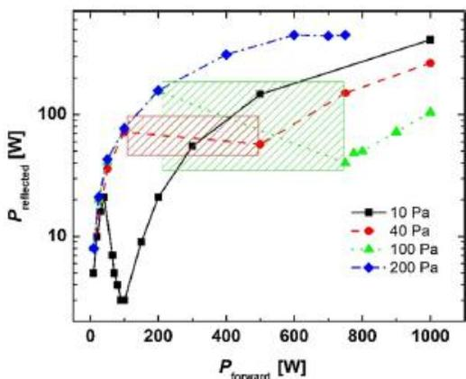
Fig. No. 04: Dependence of the reflected power for different pressures on forward power of the RF power supply
