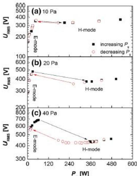
Fig. No. 08: Dependence of the Urms values on the power deposited to the plasma for different pressures: (a) 10 Pa, (b) 20 Pa, (c) 40 Pa. Measurements were made for an increase of the power given by RF power supply (increasing P<sub>a</sub>) and after that, a decreasing power (decreasing P<sub>a</sub>) in order to detect hysteresis
