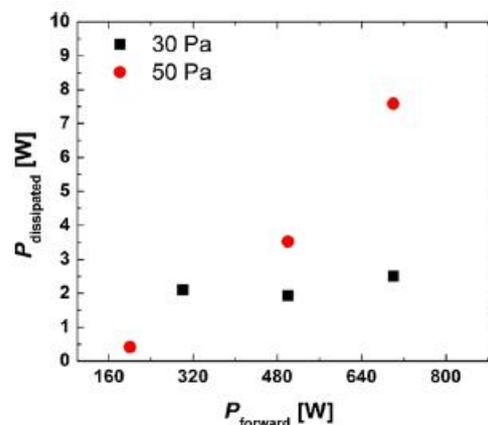
Fig. No. 03: Power dissipated as coil heating for two different pressures while plasma was ignited
