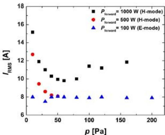
Fig. No. 06: RMS current values shown as a function of working pressure
