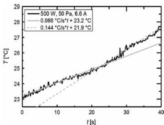
Fig. No. 02: Time dependence of the coil temperature after the plasma ignition
