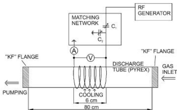
Fig. No. 01: Experimental set-up for the ICP RF discharge
