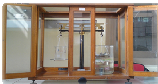
Fig. No. 01: Mucoadhesive Strength measurement modified balance
