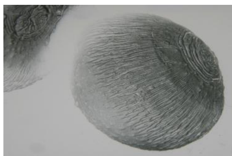
Fig. No. 01: SEM photomicrograph of uncoated alginate beads.
